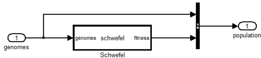
Fig. 5 – subsystem ( Fitness function ) creating structured output signal
