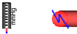
Figure 5.6: From left to right: Pressure sensor provides transformation from hPa ( N \cdot cm^{-2} ) to mmHg , PressureFlowConnector provides connection of pressures and flows between components.
