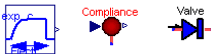
Figure 5.13: Components of VAD pump – from right left to right driving pressure, variableCompliance and valve
