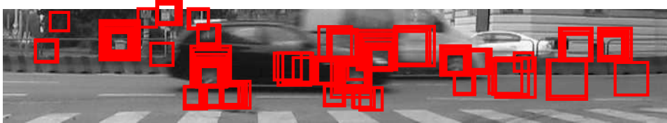
(a) Multi-scale detection of single wheels (size of squares denotes scale of detection)
