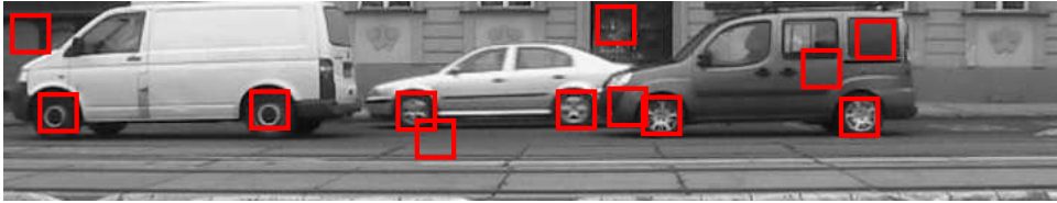
Figure 2.8: Wheel detections after thresholding and NMS. The detection was run on scale = 1, i.e. the size of the squares is 20 pixels.
