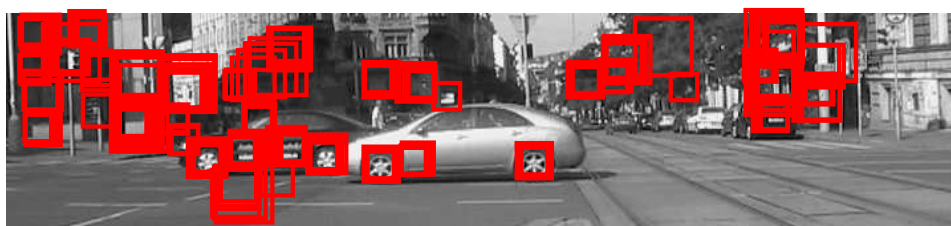
(a) Multi-scale detection of single wheels (size of squares denotes scale of detection)
