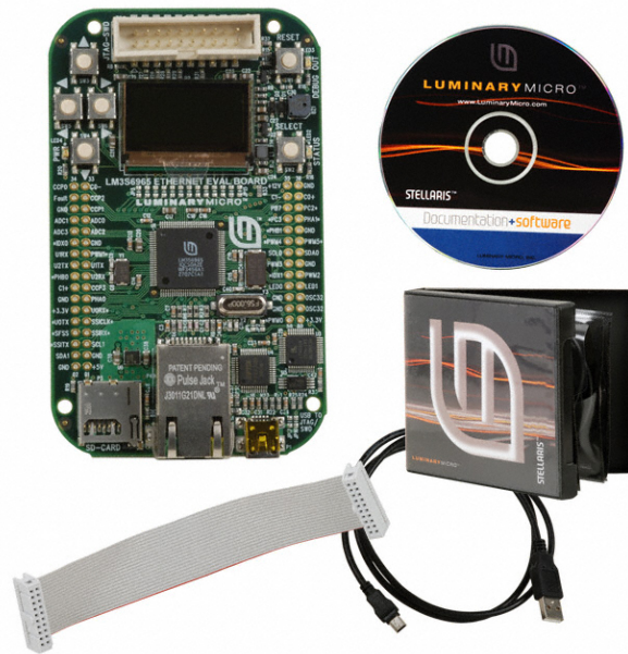
Figure 33: Control Board is based on LM3S6965.
