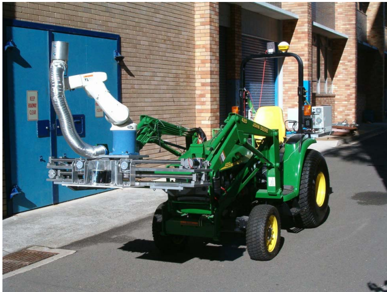
Figure 10: Fruit picking system of Zhao et al. (Source: [23])
