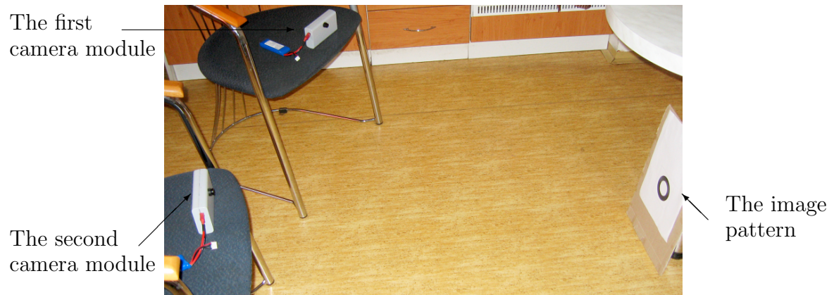
Figure 26: Camera modules tracking the image pattern during the experiment.
