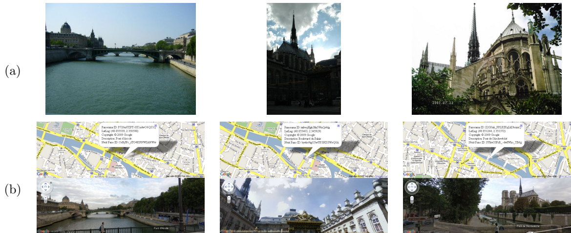
Figure 6.4: Examples of estimation the map position for a query image. (a) Query image, (b) the map including computed position highlighted by the callout with the geo location, street name and some google informations. Google street-view preview is shown below the map. This presents that we can obtain street name and panormatic view for the query image.
