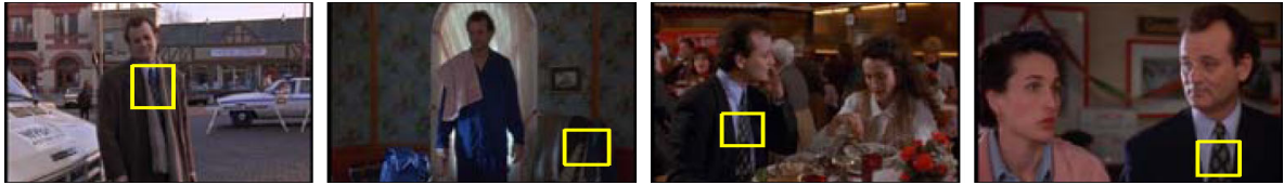
Figure 2.2: Object retrieval. Example of Video Google [SZ03] approach, shows retrieved images from the Ground Hog Day movie with highlighted tie used as the query object.
