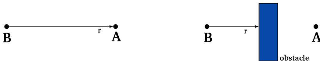
Figure 2.6. Visibility described by ray. On the left is point A visible from B because ray r can pass from A to B without colliding with another object. On the right is point A not visible from B because before reaching A , ray r hits obstacle.
