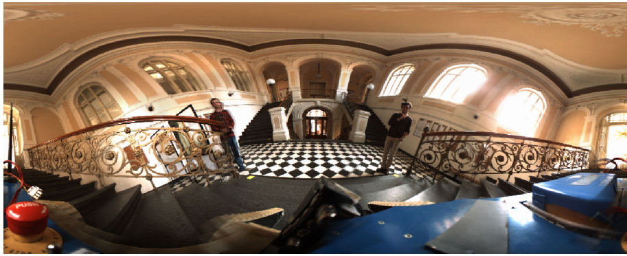
Figure 3.2: Stairs as seen from the robot omnica camera in a spherical projection.
