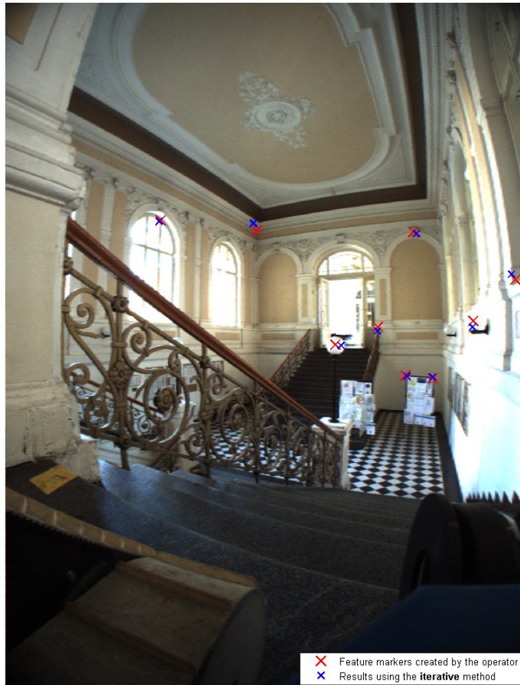
Figure 5.14. Correspondences used for calibration and their projections. Average reprojection error: 10.3, Maximal reprojection error: 19.0
