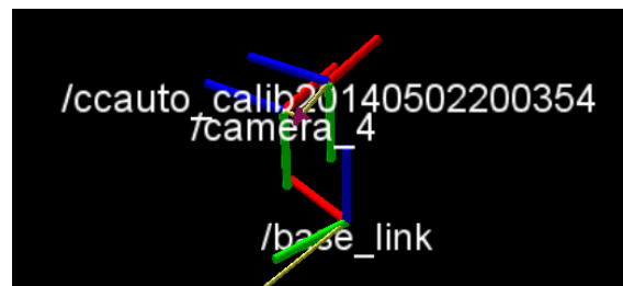
Figure 5.24. The original transform ( /camera_4 ) compared with the result of the EPnP method.
