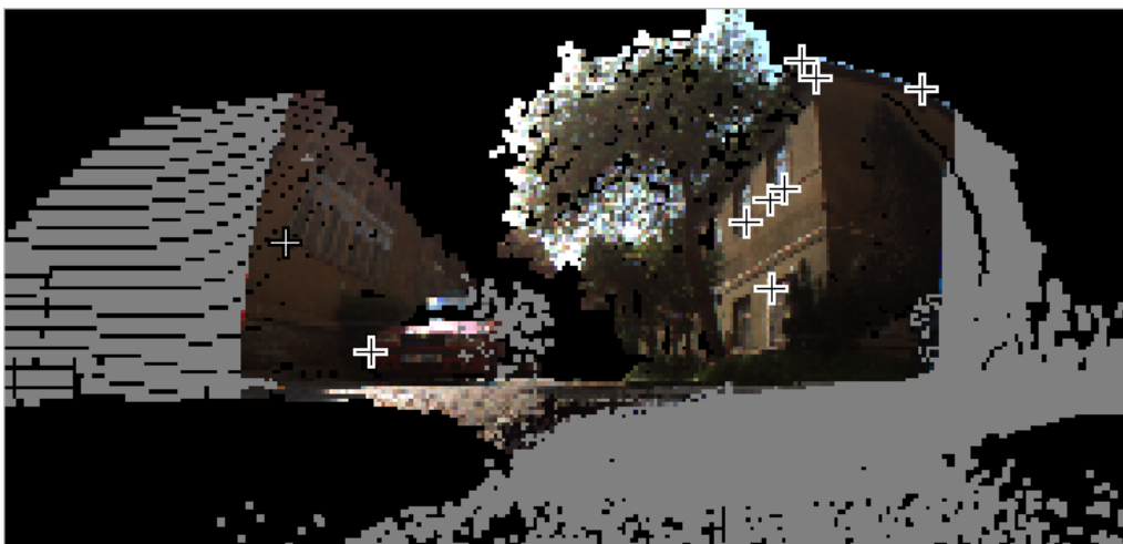
Figure 5.21. Colored range image using the calibration from the iterative method.
