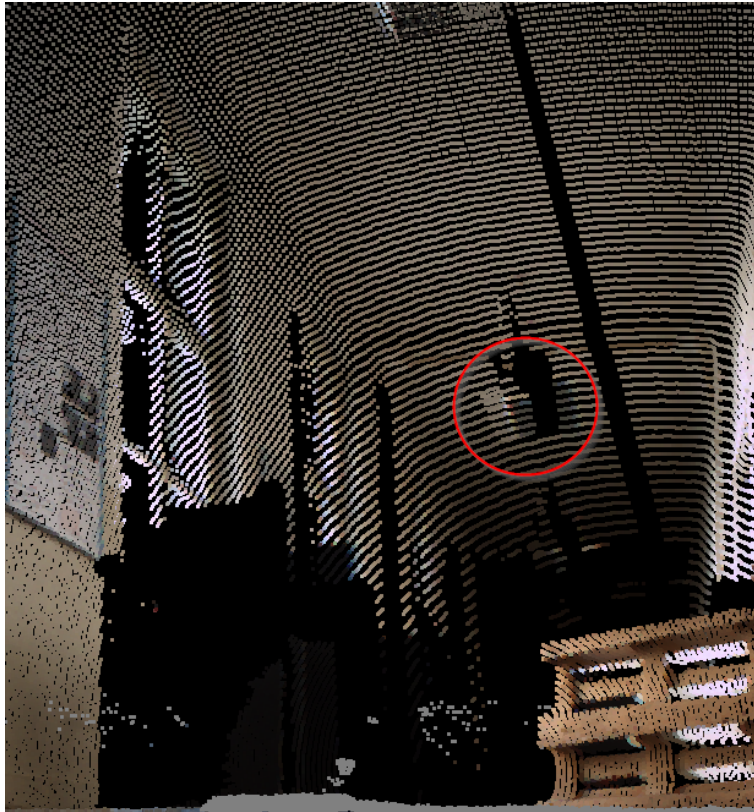
Figure 5.5. Visualization of the colored point cloud using the calibration result of the iterative method with local correction.
