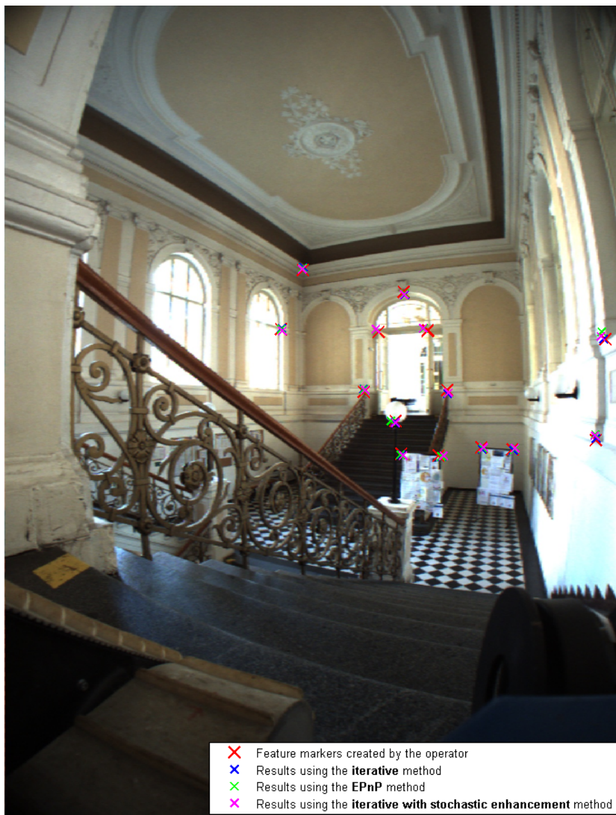
Figure 5.9. 14 correspondences used for the calibration. The point cloud density was too low to create precise correspondences on the rail.
