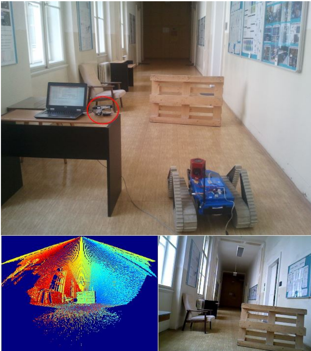
Figure 5.27. Overview of the scenario 5. Camera is sitting on the table next to the notebook. The bottom-right image is the actual image from the camera.
