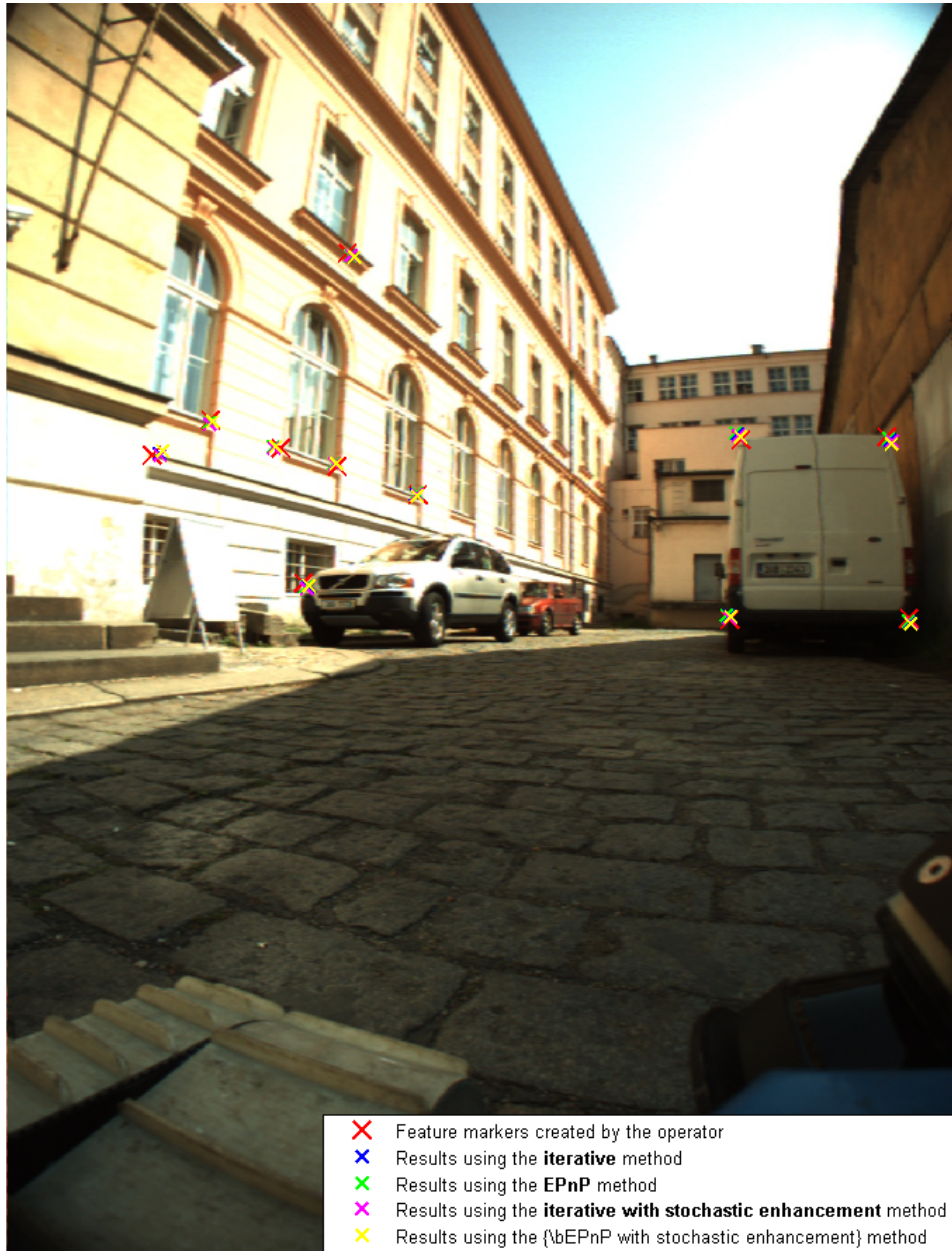
Figure 5.22. 11 correspondences used for the calibration.
