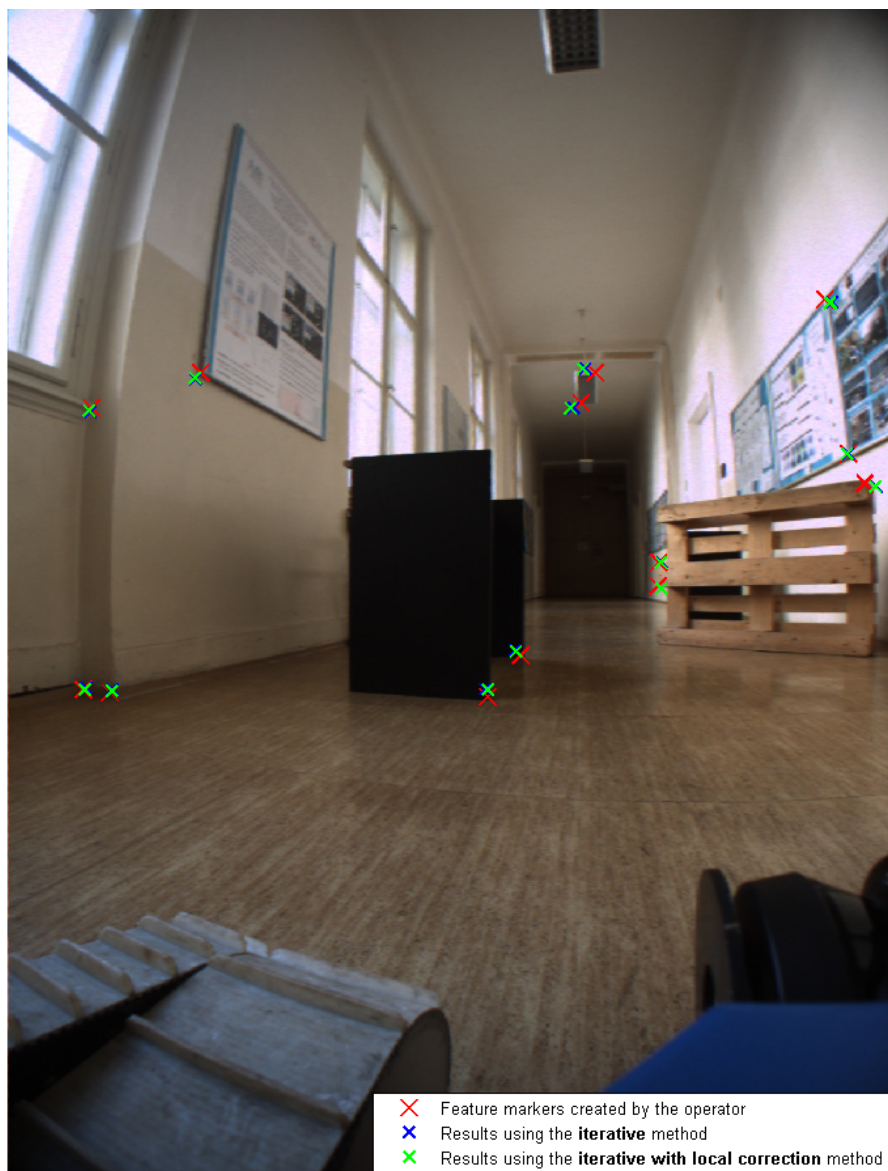
Figure 5.2. 13 correspondences used for the calibration.
