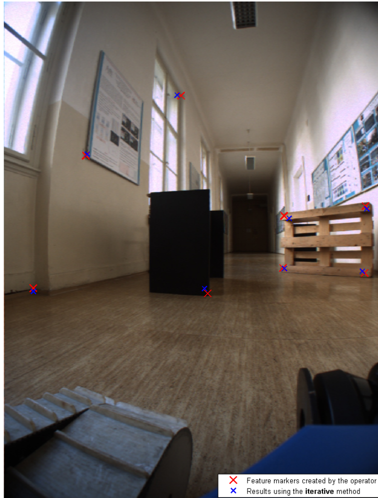
Figure 5.7. Correspondences used for calibration and their projections. Average reprojection error: 11.6, Maximal reprojection error: 19.0
