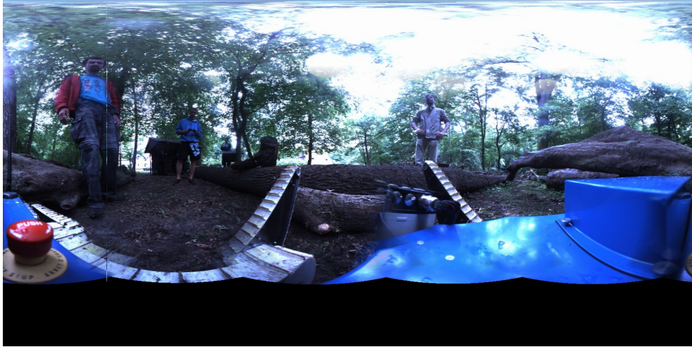
Figure 4.8: Krč Forest scene captured by the omnidirectional camera. The robot traverses three times the log that is visible in the center of the image.
