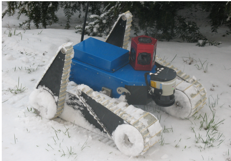
Figure 1.1: NIFTi robot. The omnidirectional camera used in this paper is mounted on top of it (painted in red).
