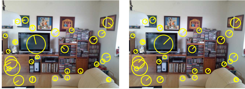
Figure 3.1 A visualization of standard SIFT keypoints on the left and upright on the right. The yellow circles represent individual keypoints. The scale of a keypoint is illustrated by the radius of its respective circle and an orientation by a line going from the center of the circle to a point on it. This example shows only keypoints of a scale higher than 10 to enable a nice visualization.
