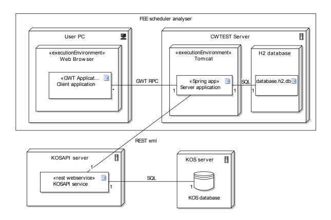
Figure 5.1: Deployment diagram showing structure of project
