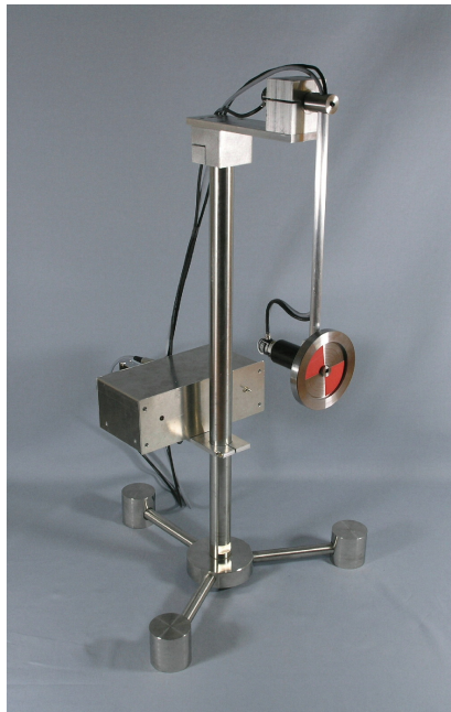
Figure 1: Laboratory model of the reaction wheel pendulum. Available from [16]
