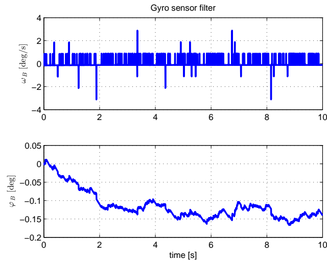
Figure 17: HiTech NXT Gyro Sensor in a motionless state with calibrated offset and filtered drift.
