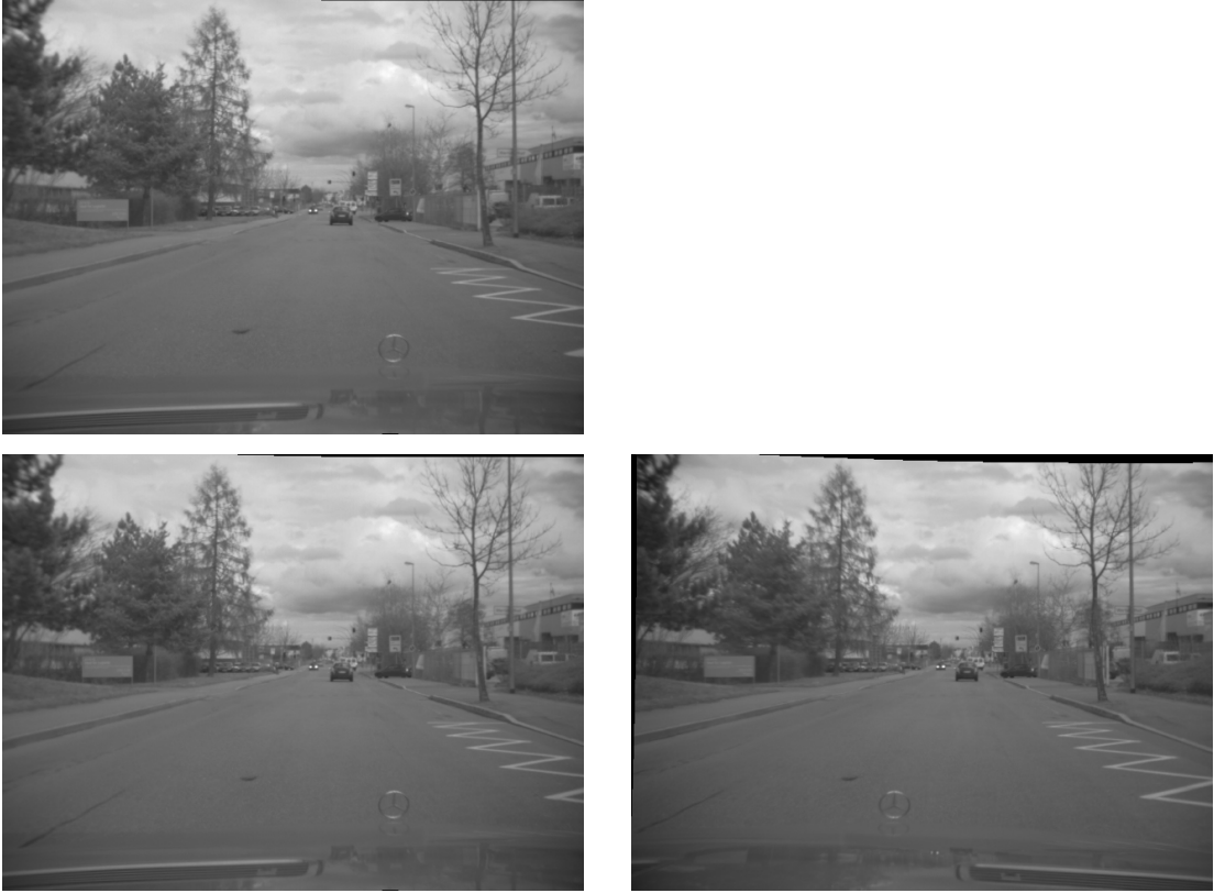
Figure 5.1 Cameras' setup used in this experiment. Bottom row: a pair of horizontal images. Left column: two consecutive images from left camera are used to obtain a pair of forward motion images.
