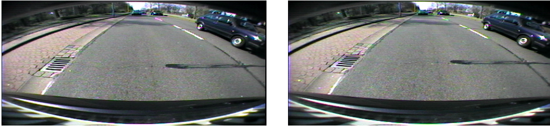
Figure 5.12 Original input images obtained by reversing camera. The camera was found to closely match a perspective camera model with radial distortion.
